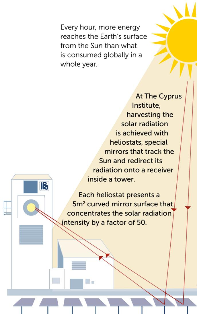
Our field of heliostats at the PROTEAS facility on the southern coast of the island yields an intensity of 2,500 suns, reaching temperatures in excess of 1,000°C. The sunlight is converted into heat, which is stored for later use in a tank filled with high temperature molten salt. This means the solar energy can be used anytime, on cloudy days and at night. The stored energy is used for the co-generation of electricity and desalinated sea water.
